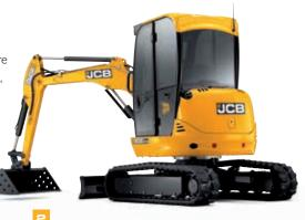
Good size door width for easy access and the door itself latches back within the tailswing so you can work with it open. To make access even clearer, the left control pod hinges up and we have removed the left foot pedal (a changeover switch on the joystick allows you to control right and left pedal operations with just the right pedal).
