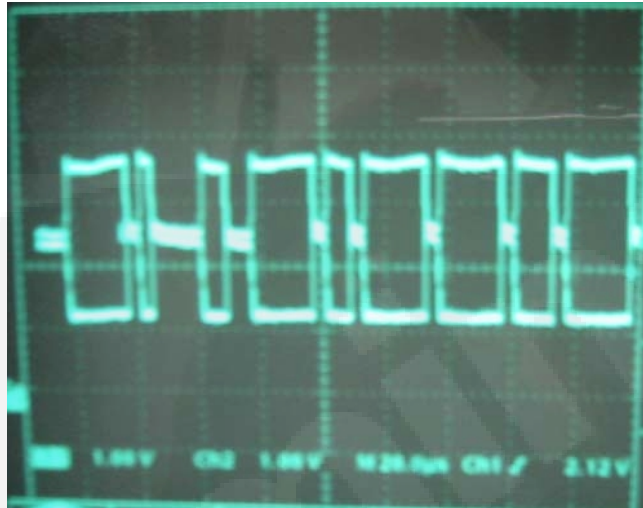
FIGURE 6. CAN DATALINK: GOOD SIGNAL
