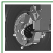
TX1053406A-UN: Replace Wheel Hub Oil
