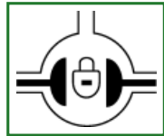
TX1052887-UN: Manual Differential Lock Indicator
