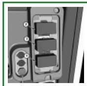
TX1082513A-UN: Fuse and Relay Boxes
