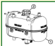
TX1082883-UN: Engine Coolant Surge Tank
