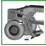
TX1051924A-UN: Four Grease Points Total—2 Per Side
