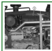
TX1083247A-UN: Exhaust Filter Location
