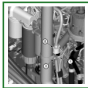
TX1086054A-UN: In-Line Fuel Strainer
