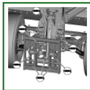
TX1051943A-UN: Balderson™ Style Front Lift Group—10 Grease Points
