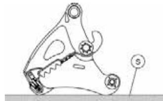
2. Ensure the coupling pins (G) are retracted as shown in the diagram.
