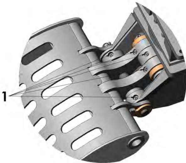
Picture 4: Lubricating pivoting points
