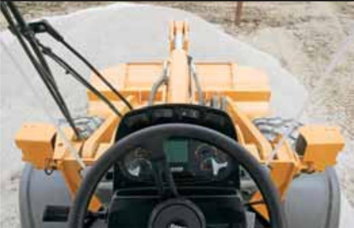
Case E Series wheeled loaders benefit from a greatly enlarged operator's cab, with up to 15 % more floor area. The tapered design is longer and wider than the D Series, offering more internal space for the driver and reduced noise levels that are among the quietest in the industry.
