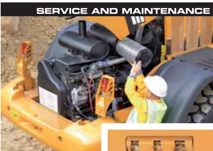
Thanks to the mid-mounted cooling module design, the engine sits at the rear of the machine, where it contributes to the counterweight. A single-piece electrically-operated engine cover lifts clear of the engine for service and maintenance, and all daily checks can be easily reached from ground level, with fluid sight gauges on all reservoirs.
