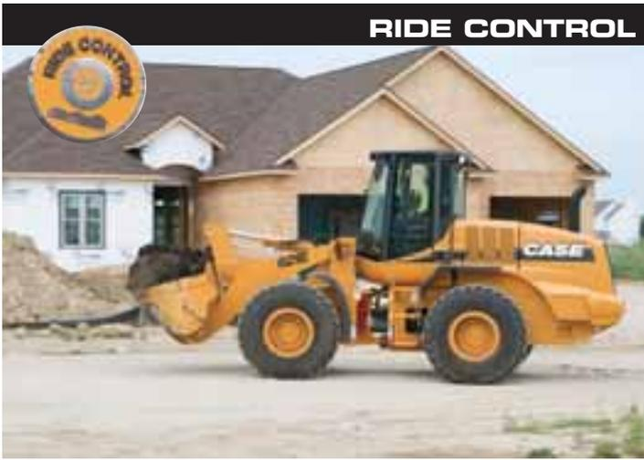
Load retention and cab comfort can be further improved with the addition of optional Ride Control, a system that allows the lift arms to float when the machine is moving, preventing bounce in the cab and at the wheels. Ride Control permits higher travel speeds during load and carry operations, reducing fatigue for the operator and increasing productivity.
