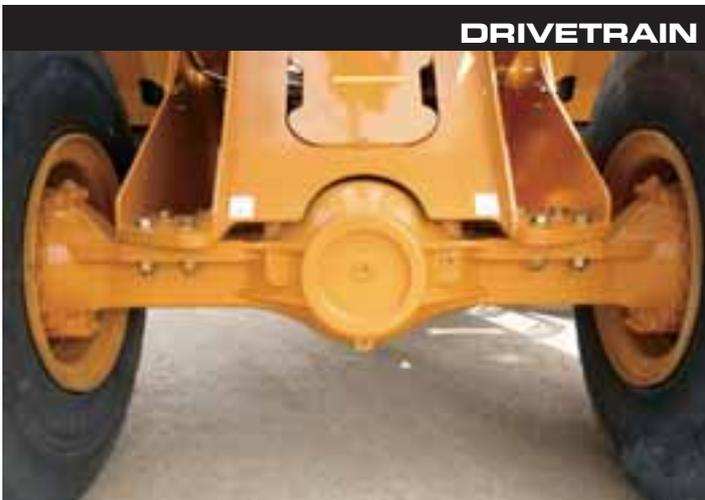
The 621E wheel loaders use a torque sensing autoshift transmission with four forward gears and three reverse ratios. Top forward speed is 38.6 km/h.
